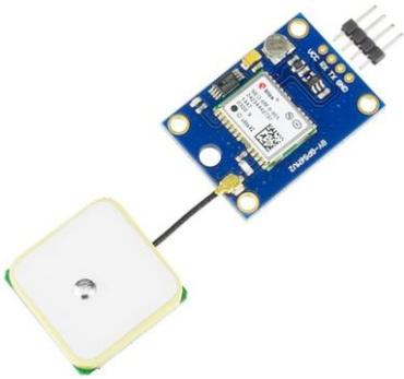
GPS Module – The one shown has a separate antenna (The white ceramic square) and the receiver, mounted on a breakout board, ready to have the header pins attached
