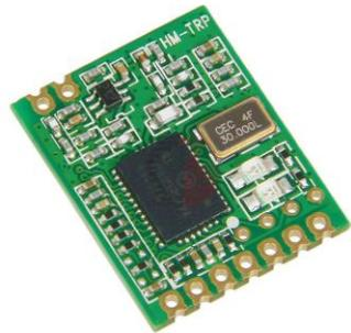
LoRa Transceiver – Again with header pins provided. These pins will be used initially to program the frequency of the LoRa via USB, but will operationally be used for +voltage, -voltage, transmit (TX) and Receive RX) data
