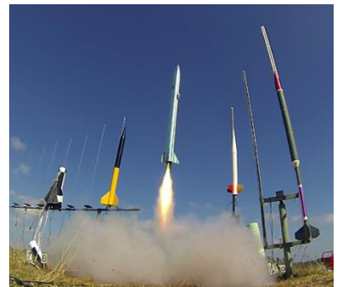
Michael's "Jedi" on a H128. Ben's V2 (on the left) shows the result of a motor CATO
